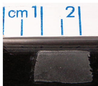
Figure 6. Polymer film containing vertically aligned SWNT. Film thickness is roughly 1 mm.
